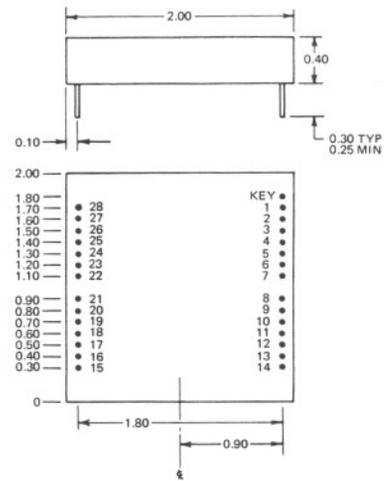
**PIN CONNECTIONS (TOP VIEW)**
